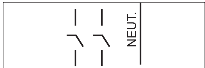
Three-wire SN, 120/240 Volts ac, No Fuse
