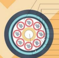
Wide range of designs, both metallic and dielectric, incorporating filled buffer tubes. Available metal-free or armoured design and also dry core or jelly filled.
